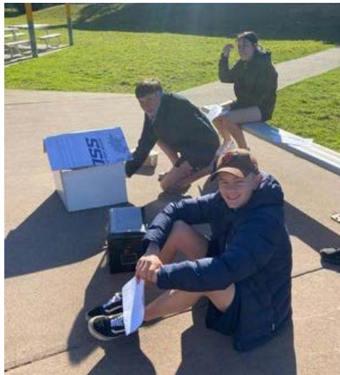
Students recording temperatures using infrared thermometers. Houses were placed in the sun for 20 minutes and then moved to the shade for 10 minutes to determine whether their houses successfully meet the design brief.
