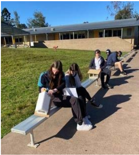
Students recording temperatures using infrared thermometers. Houses were placed in the sun for 20 minutes and then moved to the shade for 10 minutes to determine whether their houses successfully meet the design brief.
